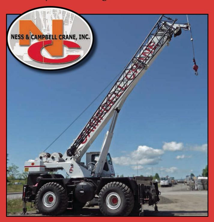
Boom Lengths: 35' to 110' Jib Lengths: 33' to 58'
